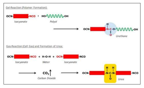
Figure 1-2: Simplified basic reactions of polyurethane formation.
