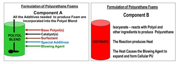
Figure 2-1. Chemical constituents required for moulded polyurethane production reaction.
