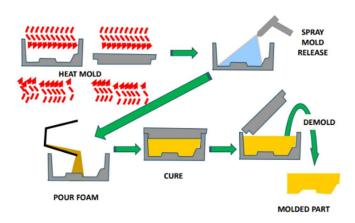
Figure 2-2: Visualizing the moulding process
