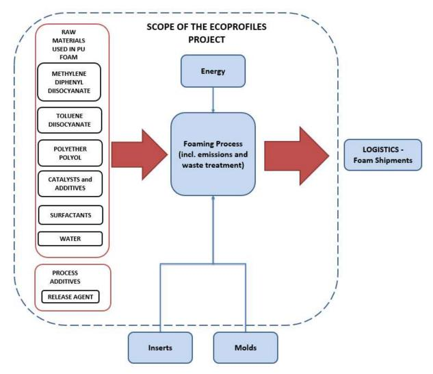
Figure 2-3. Cradle-to-gate system boundaries (moulded PU foam).
