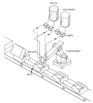
Figure 1-1: Process of moulding PU foam Source: Flexible Polyurethane Foams, Dow Polyurethanes, 1997
