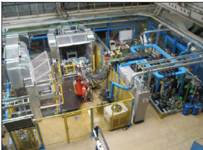
Fig. 12. Photo of a reaction injection molding system for production of automobile seats; manufacturer: Cannon (company photo: Bayer Material-Science)
